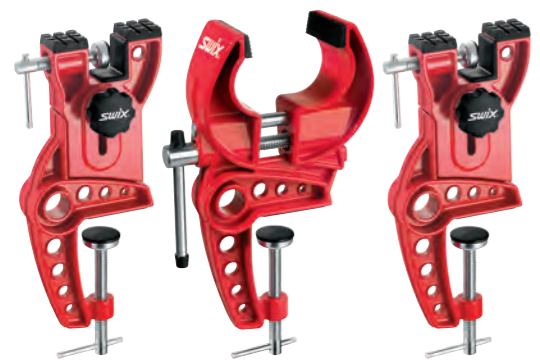
T0149-50 WORLD CUP SKI VISE Swix three piece vise with 50 mm wide jaws. Opens from 40 mm to 100 mm, for better grip and stability when working on carving skis and radial alpine skis. Two angles for side edge position; 60 degrees and 90 degrees. 60 degrees gives better control for side edge work. Ea.
