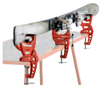
T0149-20 JAW ECONOMY VISE Three pcs. vise with jaw fixation. 20 mm wide jaws. Opens from 35 mm to 90 mm. 60 and 90 degrees side edge working position. Light weight and compact. Ea.
