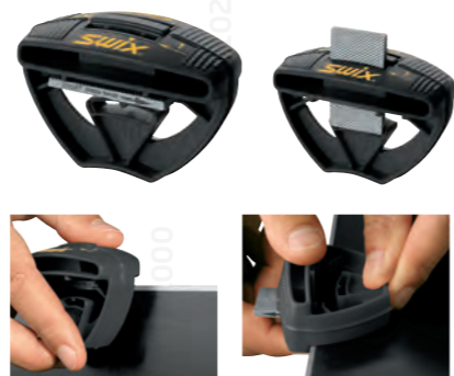
TA3001XF Pocket size file holder with file included for sharpening steel edges. Double function: 1) Side edge 88° and 89°, and 2) Base edge 0.5° and 1°.
